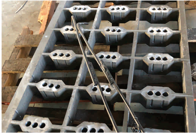
Holes to lighten the whole mould
